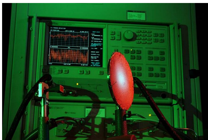
The free-space measurement of transmission and reflection at 75-110GHz.
