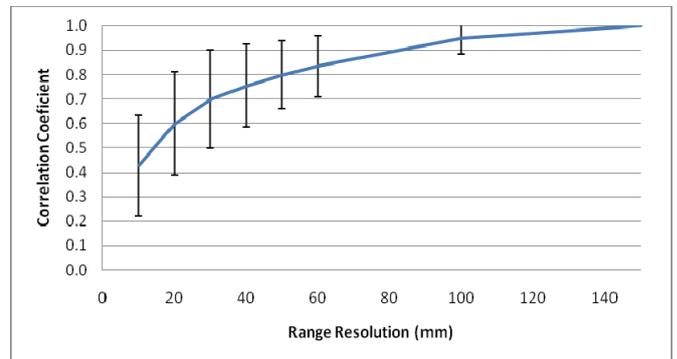
Figure 4: Correlation Coefficient between Range Profiles Separated by 1° in Azimuth.
