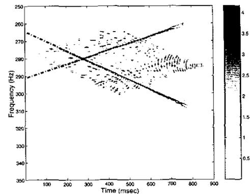
Fig. 7. A section of the Wigner distribution showing the crossing chirps and the detected chirps superimposed
