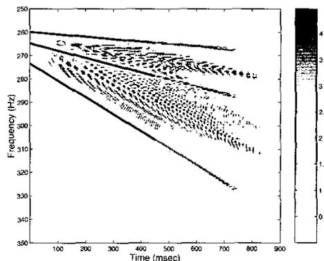
**Fig. 4.** A section of the Wigner distribution of the actual chirps with the detected chirps superimposed as dotted lines
