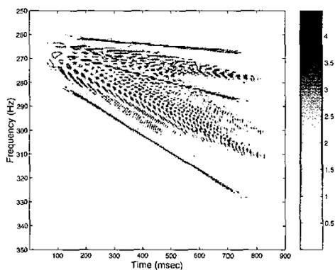
**Fig. 3.** A section of the Wigner distribution showing the three chirps
