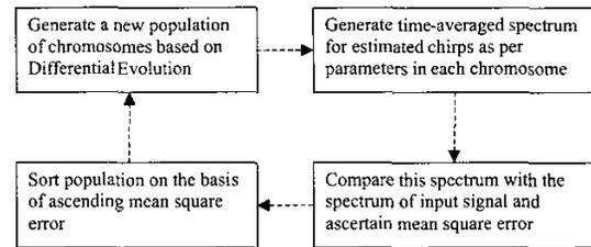
Fig. 2. Schematic block diagram of the algorithm for chirp detection and parameter estimation
