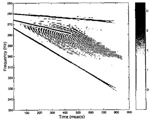
Fig. 6. A section of the Wigner distribution when chirp amplitudes are 1,0.15,1 with the estimated chirps superimposed
