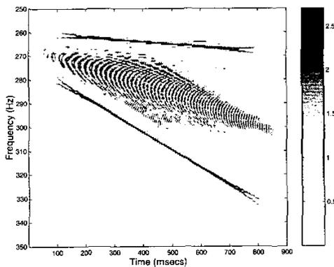
Fig. 5. A section of the Wigner distribution when chirp amplitudes are 1,0.15,1 respectively
