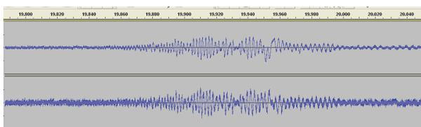
Figure 9: I/Q channel radar data on the transit of a suspected Pipistrelle bat through the radar beam. An amplitude modulation with a periodicity of approximately 47ms is clearly seen.
