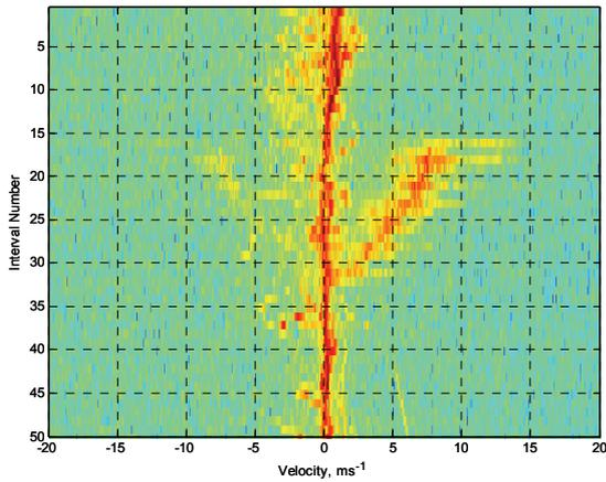
Figure 5: Short Time Fourier Transform of Peregrine on a radially inbound trajectory that passes over the top of the radar. The horizontal axis is the radial velocity measured from the Doppler information and the vertical axis are individual FFT time slice intervals. Each time interval is over a CPI of 100ms and there is no overlap of the CPI windows in time.
