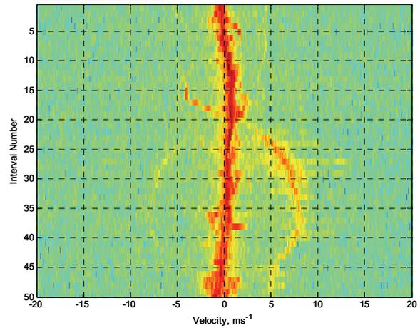
Figure 4: Short Time Fourier Transform of Peregrine on a crossing trajectory in front of the radar. The horizontal axis is the radial velocity measured from the Doppler information and the vertical axis shows individual FFT time slice intervals. Each time interval is over a CPI of 100ms and there is no overlap of the CPI windows in time.
