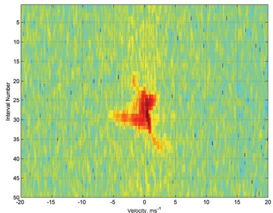
Figure 8: STFT image showing data recorded from a Serotine bat flying horizontally through a vertical radar beam. Each interval on the vertical axis is of 10ms sample duration with an overlapped CPI per interval of 50ms.
