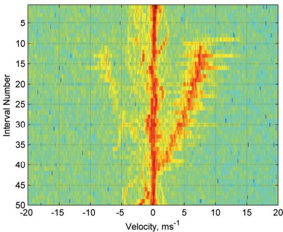
Figure 6: Time-velocity spectrogram of data imaged with 50ms per interval showing takeoff and then the Peregrine passing over the top of the radar.
