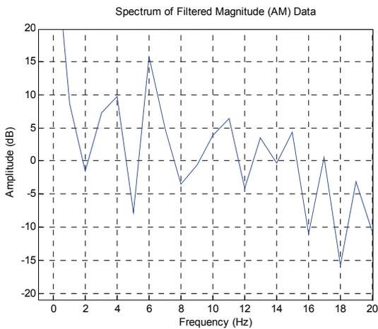
Figure 3: Spectrum of the amplitude modulation on the radar data corresponding to the Peregrine flight trial.
