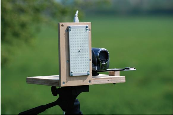
Figure 1: A K-MC2 radar module mounted on a tripod along with a video camera. Both the radar and video camera are aligned to share a common bore-sight.
