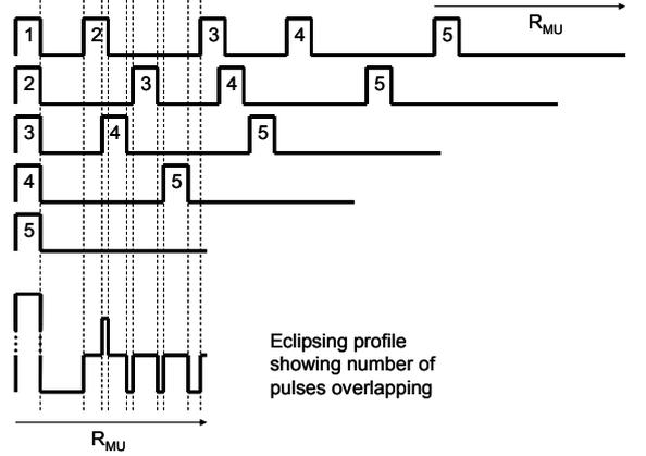
Figure 3: Generation of Eclipsing profile for example 5-pulse waveform.
