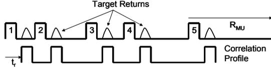
Figure 2: Range bins chosen for correlation at time offset  $t_r$  and corresponding target returns for an example 5-pulse waveform.
