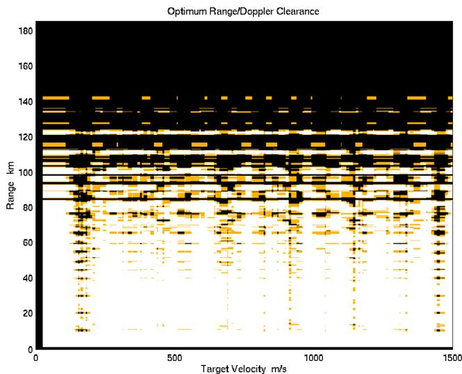
Fig. 4. Blind zone map for best 3 of 9 solution,  $5 \text{ m}^2$  target
