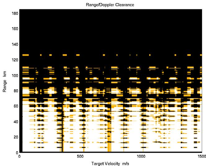
Fig. 2. Blind Zone Map of Target Returns for 8-PRF Schedule ( $2\text{m}^2$  target)
