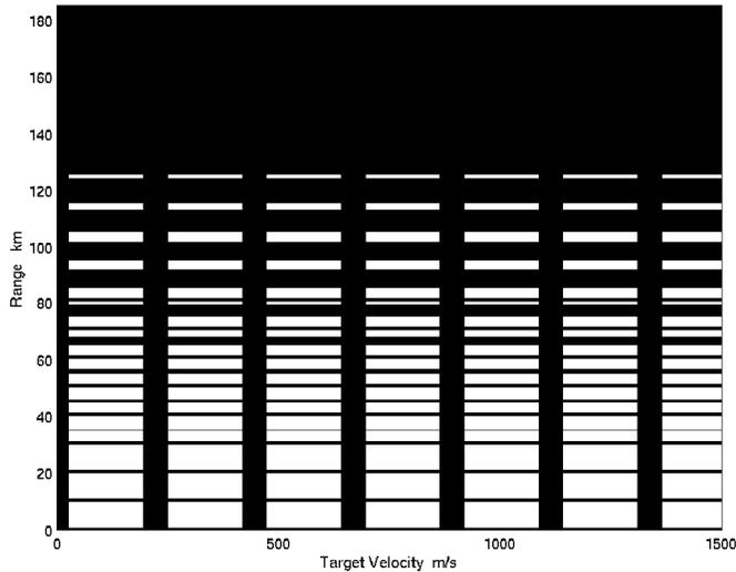
Fig. 1. Blind zones for a single, clutter limited, medium PRF waveform with PRI  $67.26\mu\text{s}$
