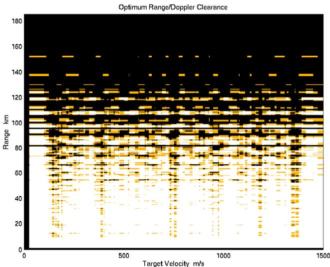
Fig. 3. Blind zone map for best 3 of 8 solution,  $5 m^2$  target
